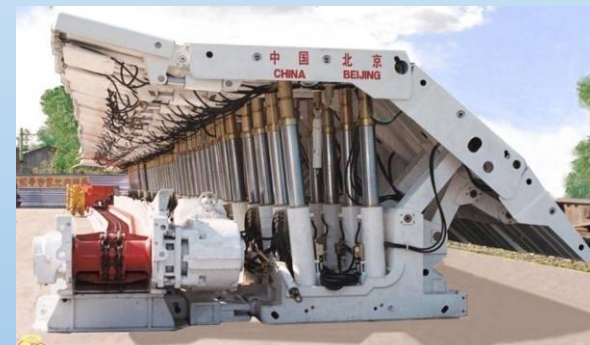
Product type of ZYP4400/16/32, the 1 st set of comprehensive coal caving equipment in Bangladesh
